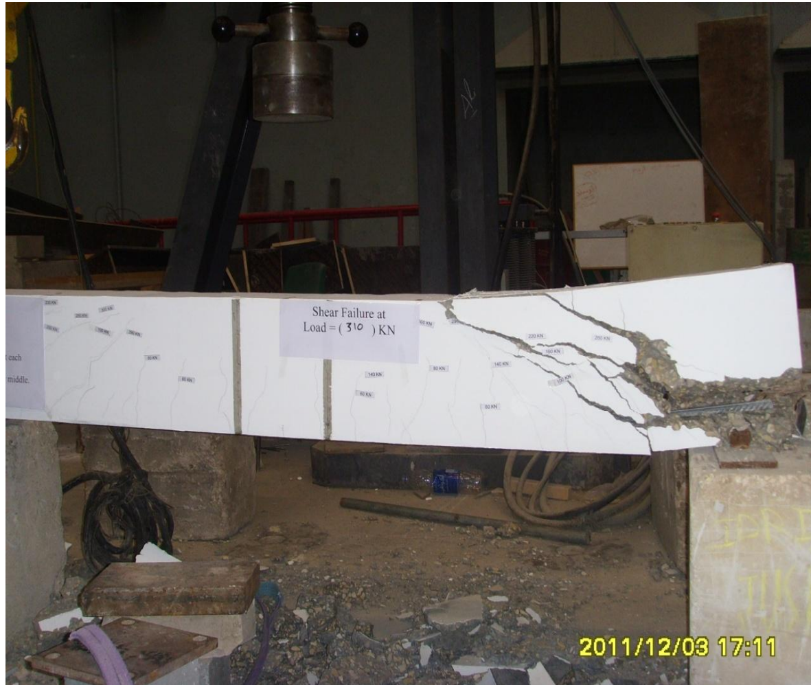
Figure 5: Beam B2, shear failure at the load of 310 kN.
