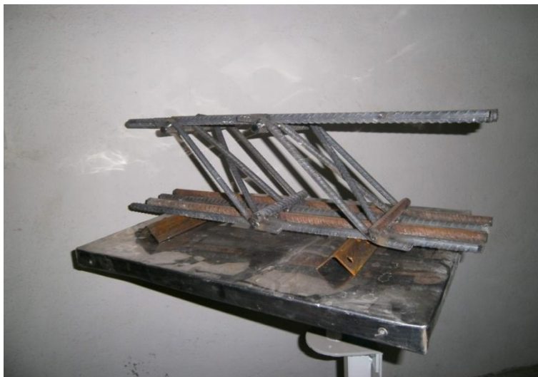
Figure 3: Rectangular swimmer bar system with cross bracings.
